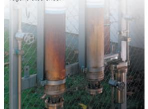
Each large cylinder is designed for a flow rate of 100 m³/h. The flow rate can easily be increased by connecting several cylinders in parallel. The various possible uses of these large cylinders call for tailor-made solutions which we will be happy to design for you.
