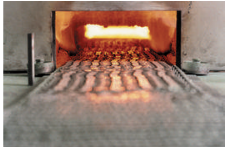
Figure 4: Sintering in conveyor furnace
