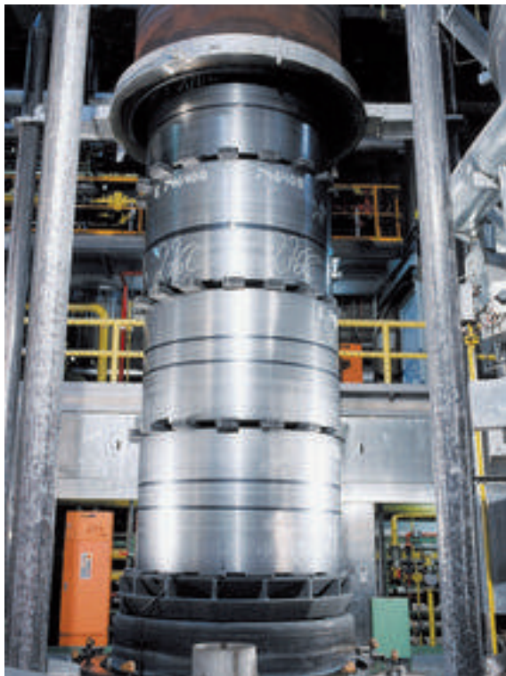
Figure 7: Coils on the floor of a bell-type furnace with high-convection technology
