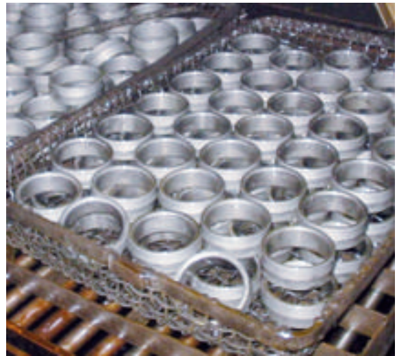
Hardening bearings after the quenching bath
