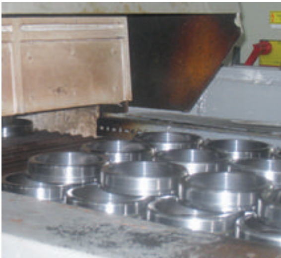
"Soft" bearing rings at the furnace entrance
